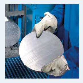
WESPA Standard bandsaw blades: Break-In-Process increases the service life of conventional bandsaw blades.
